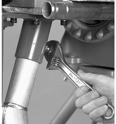
12 Release the lower legs by loosening the hex bolts. Turn the leg pads at the bottom until they rest flat on the floor.
